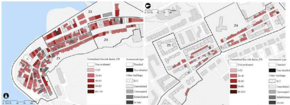
Figure 12 - Fire risk map of the urban core of Seixal, Portugal (Ferreira et al., 2016)
